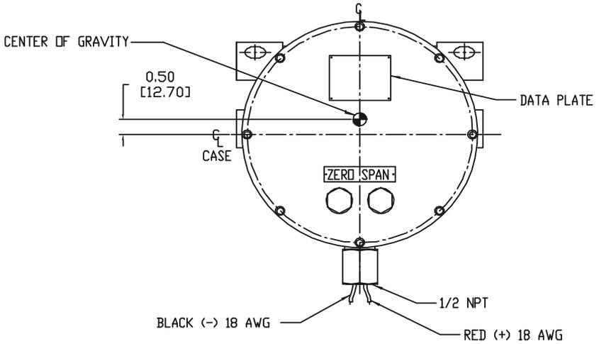
Figure 6.1—764 transmitter, front view (connector assembly not shown)
