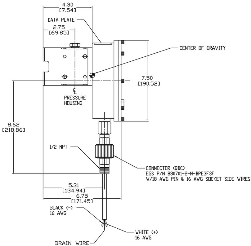
Figure 6.3—764 transmitter side view
