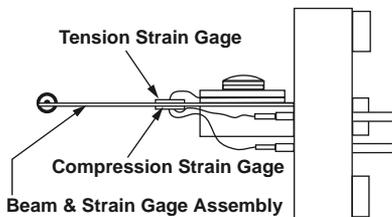
Figure 2.2—Strain Gage Assembly
