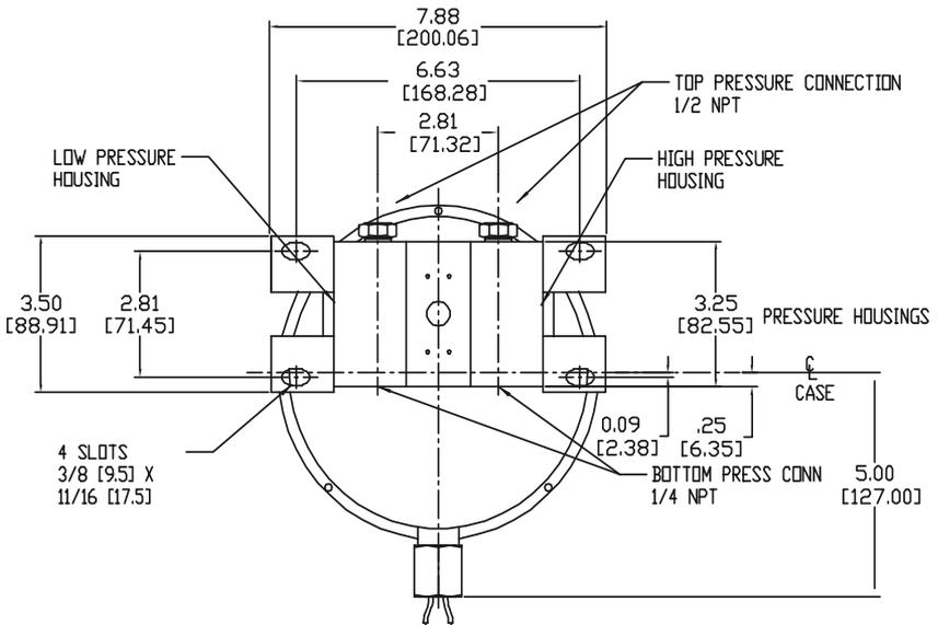
Figure 6.2—764 transmitter, rear view (connector assembly not shown)
