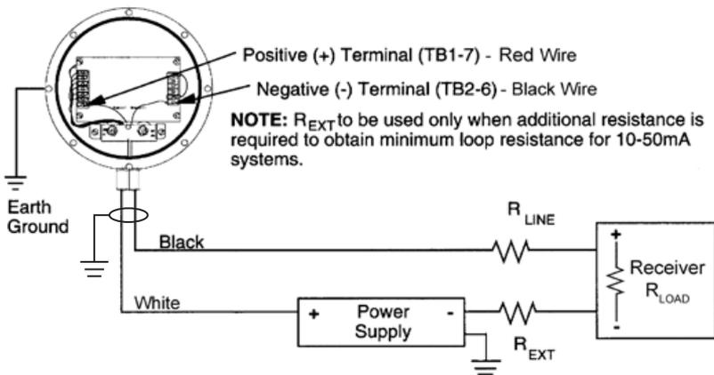
Figure 3.1—Typical field wiring connections
